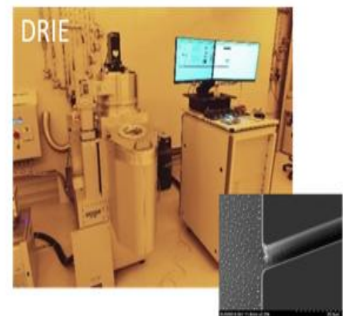
Creation of so-called hard masters for soft-lithographic processes Etching of final structures mainly into silicon (MEMS, BioMEMS)
