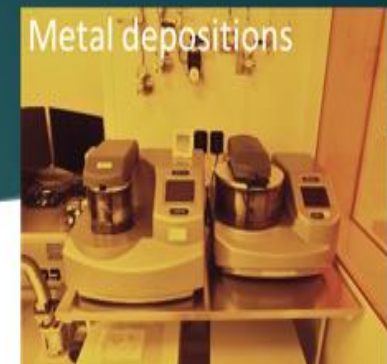
Production of chrome masks Au/Pt deposition during electrode construction Sample preparation for SEM
